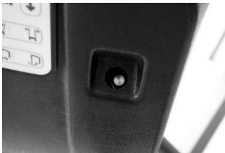
Figure 14 – Manual emergency safe lowering with the key for emergency lowering
