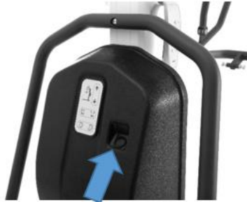
Figure 13 – Location of manual emergency lowering
